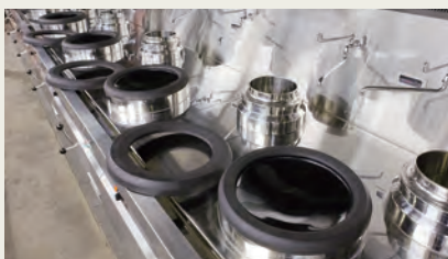
Adapter ring that can share \phi 450 \sim 600 of Chinese range by fitting and removing it. ※Patent Pending
