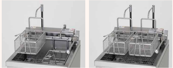
Each left and right fry baskets are lifted up individually.
